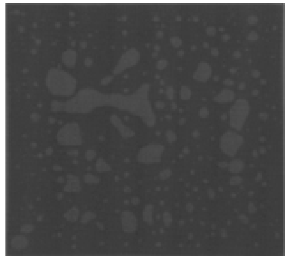
Figure 6. XRAY – Voiding P1= 300 torr, P2=P3= 0.1 torr (4.2 x 4.6mm) GaAs Die Process Per Figure 3
